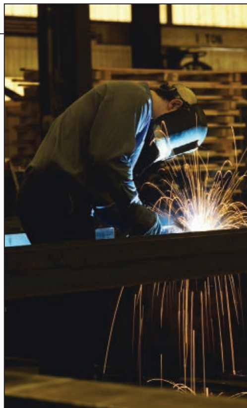
FIGURE 3. Welding shields are typically equipped with shaded lenses to protect from optical radiation
