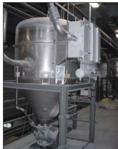
FIGURE 4. In complying with pharmaceutical and food standards, pneumatic conveyors are easy to clean with minimal product degradation
