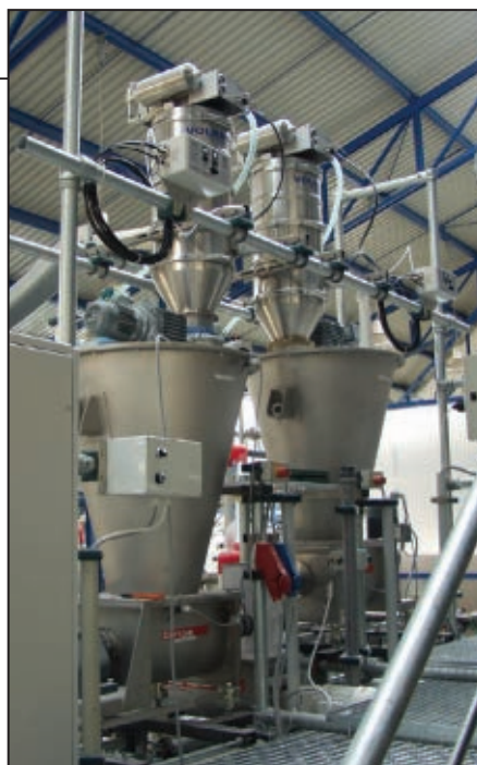
FIGURE 3. The premise for vacuum conveying is simplicity in operation, inherent reliability and hygienic transfer of material. The basic principle of this type of system is to convey the product from a feed or supply source into a delivery point suspended in a relatively uniform system
