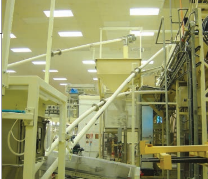
FIGURE 1. Flexible screw conveyors are the simplest and least expensive solution and can be curved to some extent, depending on the diameter
